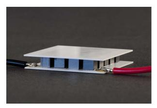
A thermal converter is blanketed on hot surfaces and can provide (extra) electric power.
