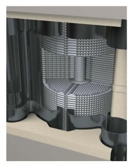
Up to 60 fuel cells are stacked in the Hexis fuel cell heating unit.
