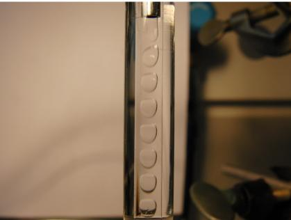
Empa's Advanced Fibers Laboratory is researching and developing active, liquid filled fibers in the «Rheocore» project.
