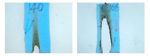
Standardised flammability tests show that organic phosphorus-containing compounds (left) provide even better protection than substances commonly used up to now, such as TCPP (right).
