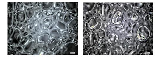
Polyurethane foam under an optical microscope - the flame retardant has no effect on the structure of the foam (left with flame retardant, right without).
